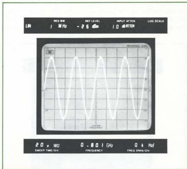
Figure 7. AM carrier demodulated in ZERO SPAN
